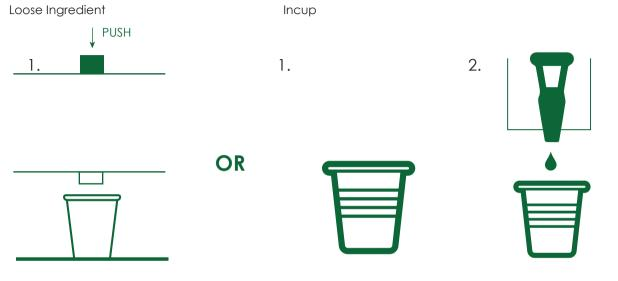
Place a suitable cup below the selected drink dispensing chute. Push the button firmly downwards For incup drinks, take a cup from your chosen drink chute (each cup is filled with the required ingredients so there is no need to add additional ingredients to the cup) Add hot water from the tap and stir
