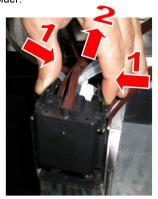
**3**▶ Remove the milk frother from the coffee outlet and disconnect Silicone tubes No. -3- and -4.
