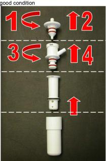
5► Disassemble the coffee outlet (1) and wash it by hand or in a dishwasher. Make sure that all the holes are free from any coffee residues , and also to use provided tools to clean the holes.
