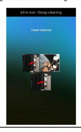
15► Wait the group cleaning ends, afterwards the machine will carry out mixer and milker cleaning cycles if present
