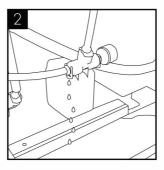
Locate the source of leakage and rectify.
