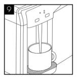
When the external cleaning (minimum 5 minutes) is completed, flush the machine using the cold button with clean water until the dispense water runs clear. Repeat briefly with the ambient button.
