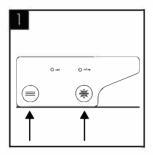
Briefly press cold/ambient dispense buttons to release internal water pressure from the machine.
