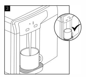
The tank is empty of sparking water when only CO2 is being released.
