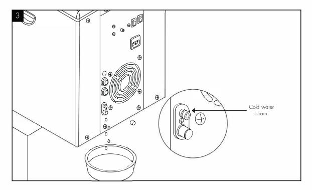
To drain the Direct Chill tank, remove the cap on the back of the machine. We recommend it is refitted immediately upon draining being completed.
