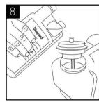
Remember to include the drip tray. If a Waste Overflow System is fitted, emply this and flush through with a small amount of sanitisation fluid if needed.
