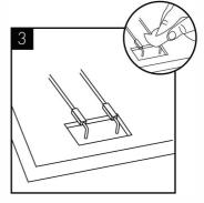
Locate the detection probe which can be found in the bottom front left hand corner. Dry the probes and internal area with a dry cloth.
