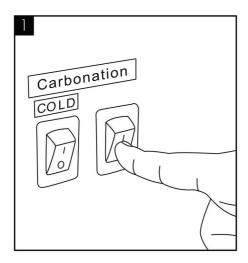
Switch off the Carbonation System switch on the back of the unit.
