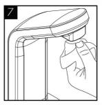
Leave the solution inside machine for sanitisation to take effect (minimum 5 minutes) while thoroughly cleaning the machine externally, pay particular attention to the dispense faucet and button controls.
