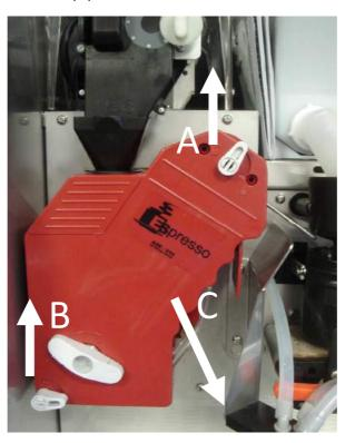
• Once the group has been removed the whole system can be cleaned with warm clean water.
