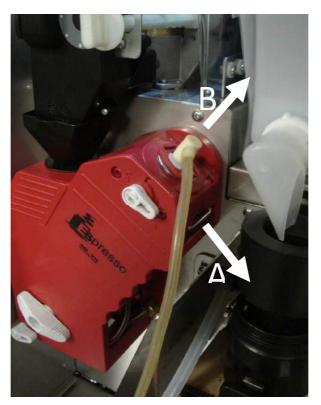
Unlock the body of the group from the machine by turning the white clips (A & B) to the
