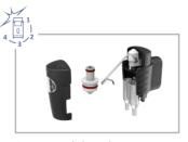
Remove and clean the steam nozzle in the milk frother. See "Removal of the milk frother"!
