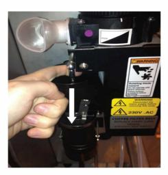
• Move the upper locking lever (C) to the vertical, (unlocked position) and remove the brew chamber assembly (D) by pulling it gently towards the front of the machine.
