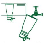
Remove canisters and dispenser mount to clean them, clean the inside of the dispenser housing and wash the dispenser mount in clean warm water, rinse dry and replace in the dispenser housing.
