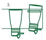
Refit the new canisters into the dispenser housing making sure that they are correctly placed.
