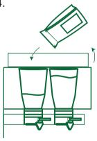
Lift lid and refill ingredient canisters as required, if empty, replace with a new canister and clean the old one.
